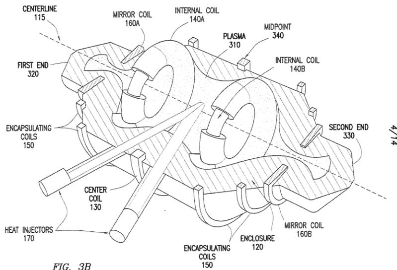
The claims all focus on the arrangement of the coils that creates a magnetic confinement of the plasma. In the patent they show what appears to be a magnetic field simulation of an implementation. It shows 3 magnetic wells, the magnetic field strength and the number of Mega amp turns (MA) of the coils.
